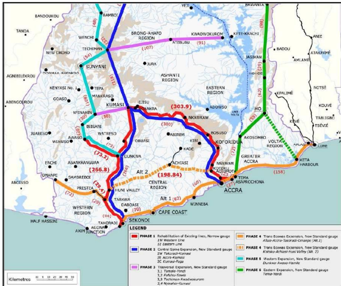
Figure 5.5: Railway Rehabilitation and Extension Plan
